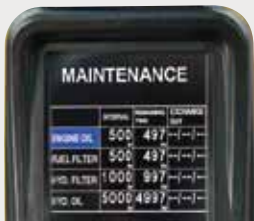
Maintenance information display
